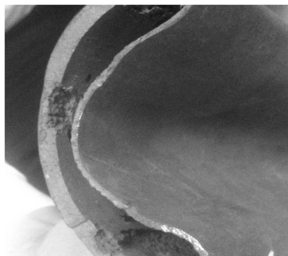
**Fig. 12. Collapsed Tubing as a consequence of uniform corrosion that resulted in low yield strength.**
