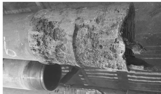
**Fig. 10. Uniform General and localized Corrosion due to CO<sub>2</sub> resulting in Metal wastage and pitting**
